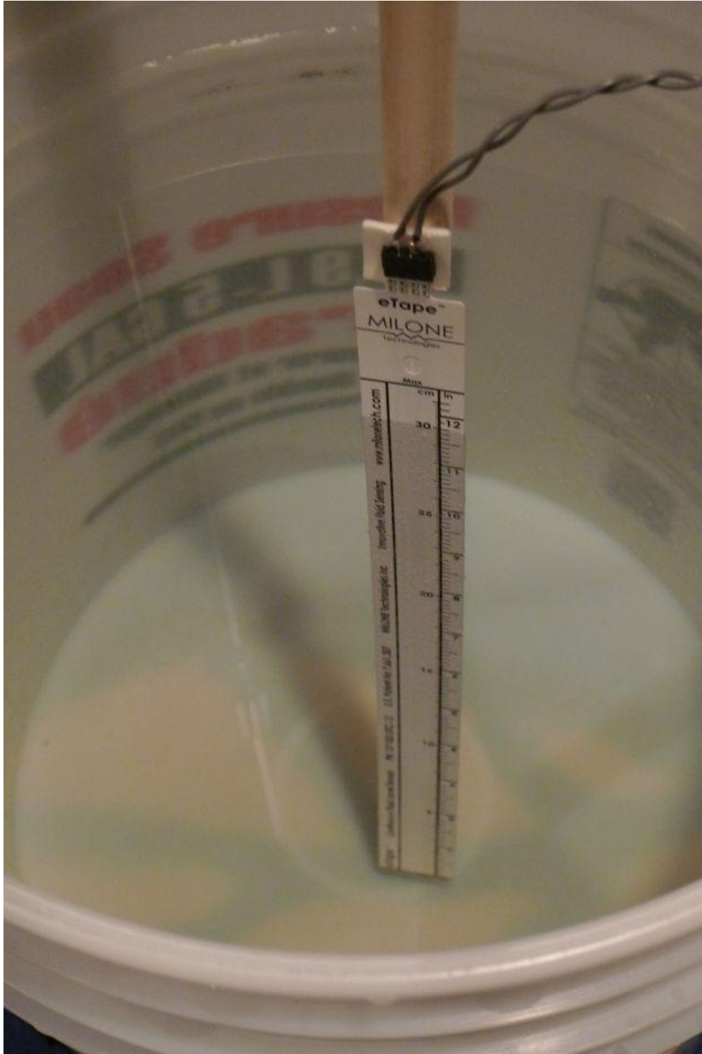
Calibration testing of tape depth sensor in 30 cm of water.
