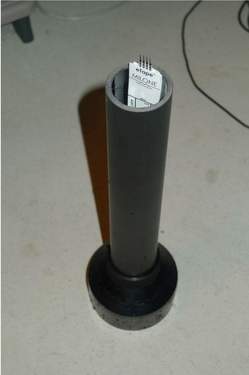
Plastic plumbing tube and coupler assembly used to make free-standing tape support, with tape sensor attached to inside top of tube. A metal sleeve (weight) was slid over this structure; the plastic floats otherwise!
